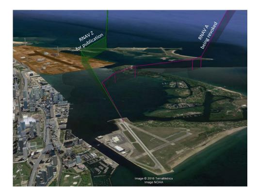
There are two new RNAV transitions over the lake that provide options for controllers to direct and sequence traffic as they prepare to use the instrument approach.
