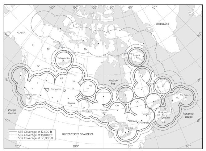
Figure 1.6.2, Secondary Surveillance Radar Coverage.
