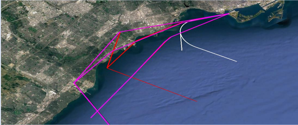
Comparison of existing (pink) and new (red and white) arrival procedures to runway 08.
