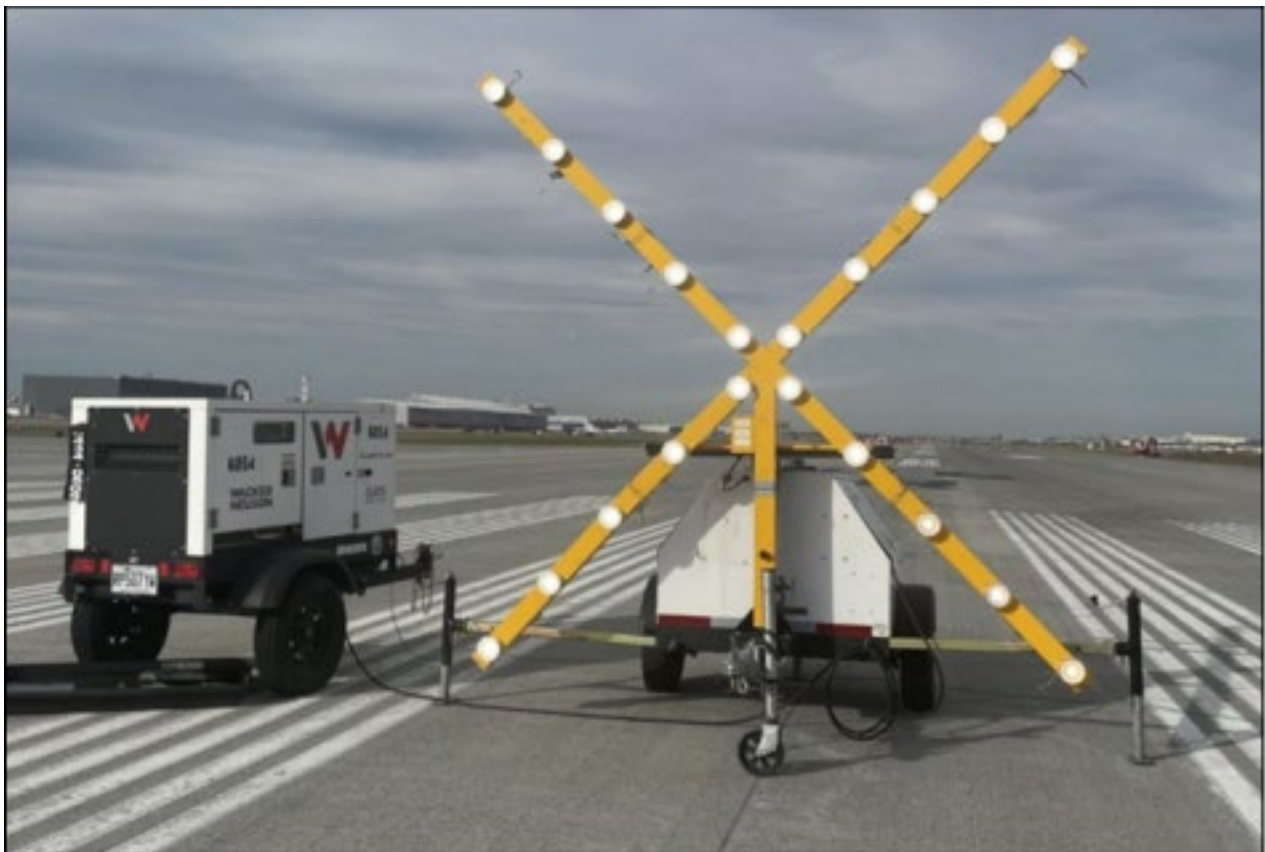
Figure 3. Illuminated runway closure “X” markers
