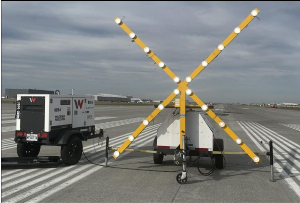
Figure 4. Lit "X" closed area markers
