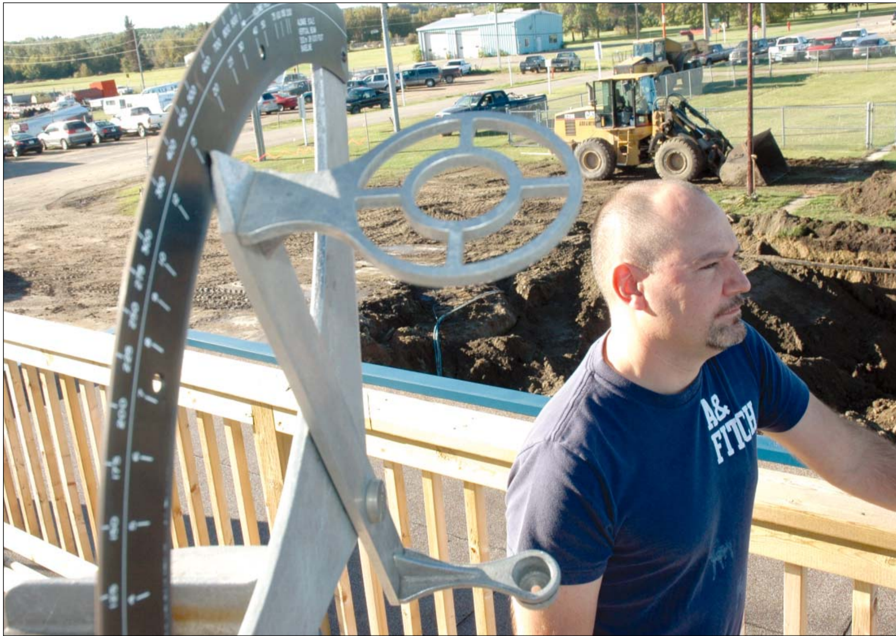
Ken Wooden, a flight service specialist and the Prince Albert airport flight service centre's supervisor, does a weather check from the observation deck. In front of him is an alidade, used to measure how high the clouds are at night. Herald photo by Joshua Pagé
