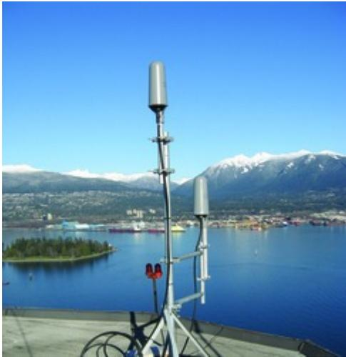
**Eleven multilateration sensors like this one have been deployed around Vancouver Harbor.**
